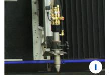
**ALFA OXYFUEL TORCH** Fast oxyfuel cutting with integrated height sensing and ignition. No probes to burn up or external ignitors to fail. Coupled with our SL-Series lifter, designed for harsh environments, let's you spend more time cutting and less time in setup. (Optional)
