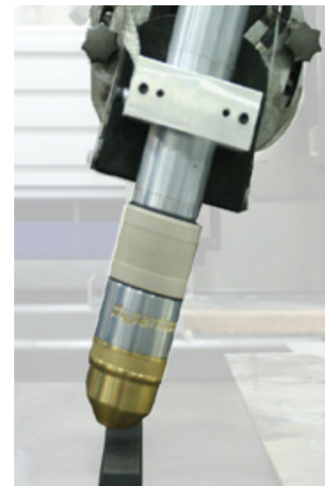
Manual Plasma Stripping Bevel Unit featured in the X-Axis. Photo shows a straight line bevel cut piece at 22\frac{1}{2}^\circ .
