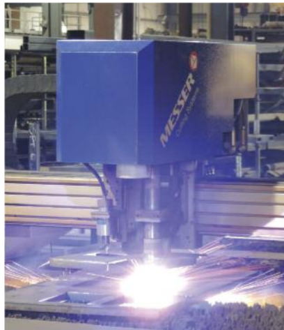
The Metal Master Plus and Hypertherm HPR260 plasma cutter from Messer Cutting Systems lets Screen Machine cut structural parts with less operator interaction.
