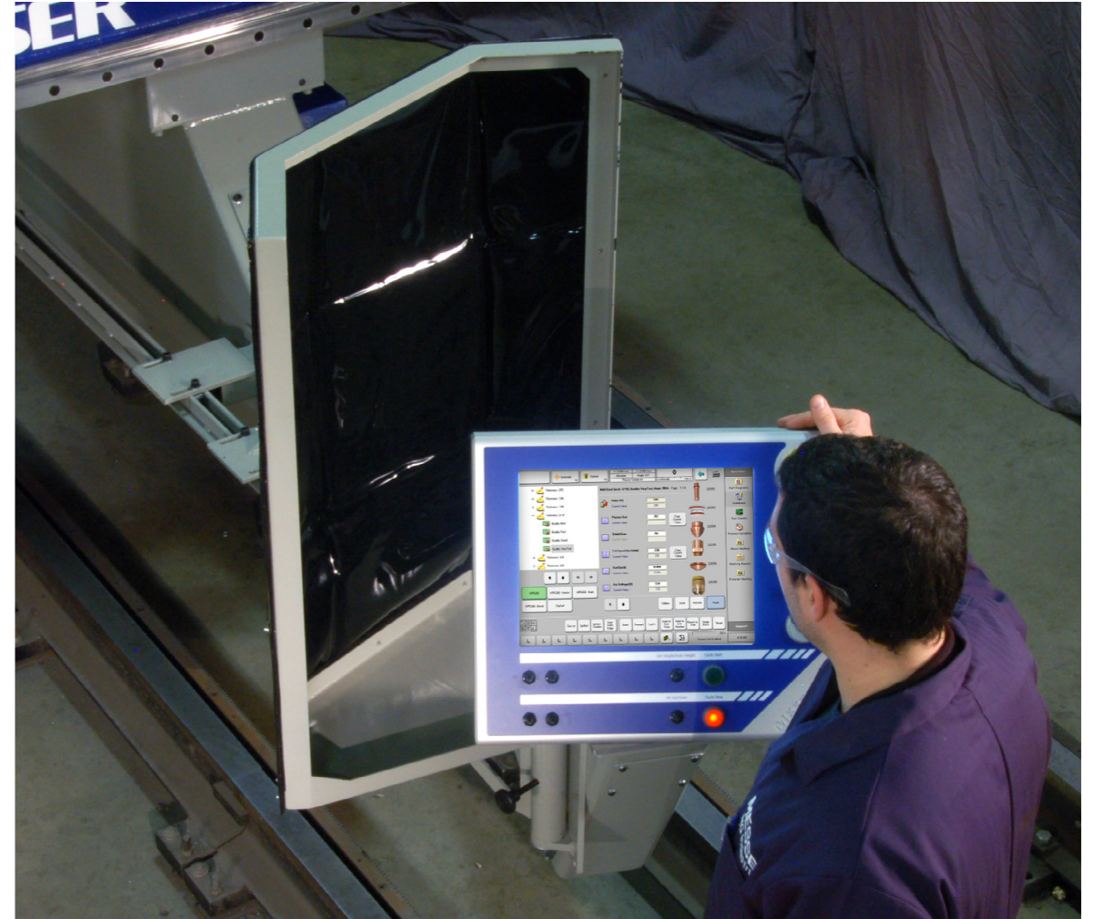
Swing away glare curtain at control station provides protection for operator.
