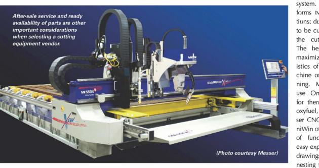
forms two distinct functions: designing the piece to be cut and controlling the cutting equipment. The best software will maximize the characteristics of the cutting machine on which it's running. Messer machines use OmniWin software for thermal cutting with oxyfuel, plasma and laser CNC machines. OmniWin offers a wide range of functions, including easy export and import of drawings and plans, and nesting for special appli-
